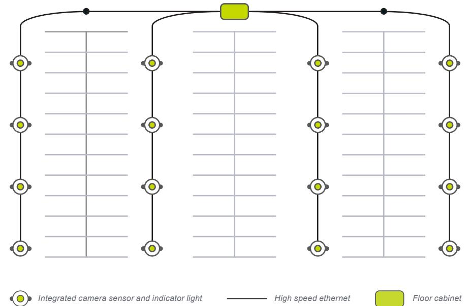
The M5 is installed above the middle of the driving lane with one unit monitoring up to 6 parking spaces.
